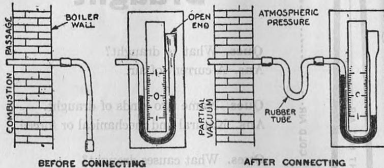
Figs. 2 and 3—U type draught gauge, at zero before connecting, and indicating 2 inches after connection. In reading, since the column in the two legs fall and rise equal distances, take the reading of one leg only and double it to obtain the draught in inches.
